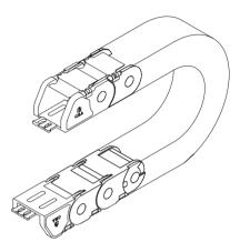
Should be attached to the both ends of the cable carrier
