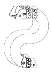
Should be attached to the both ends of the cable carrier.
